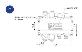
\*All measurements are in millimeters
